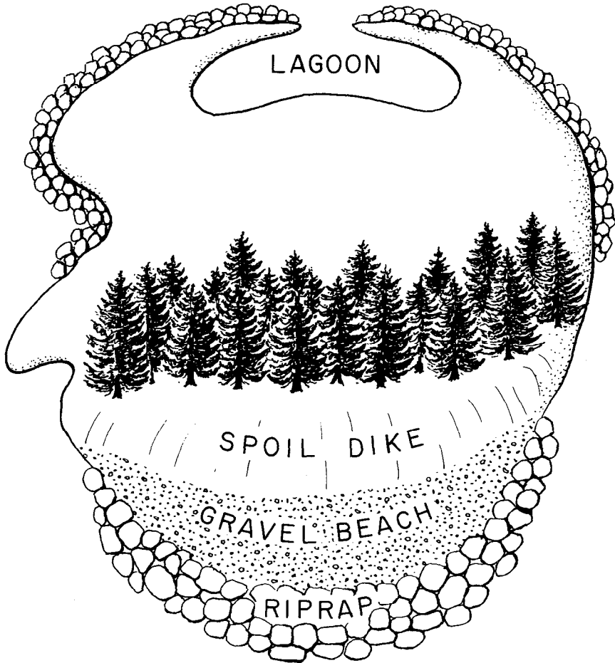
FIG. 6. Example of diked island-possible surface structure design.
