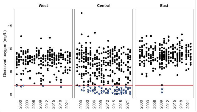
**Figure 1.0.3:** Summer (June-August) bottom dissolved oxygen (mg/L) concentrations for offshore sites by basin in Lake Erie, 1999–2023. The red horizontal line represents 2 mg/L, a typical threshold for hypoxia. Values below this are denoted by blue points.
