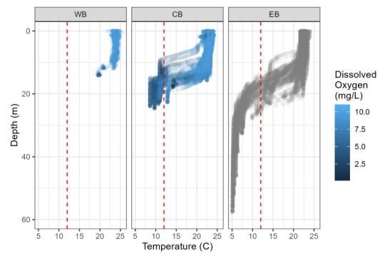
**Figure 3.0.3**: Water column profiles displayed by basin (West Basin = WB, Central Basin = CB, and East Basin = EB) with depth on the x-axis, temperature (°C) on the y-axis, and color associated with the level of dissolved oxygen (mg/L). Dissolved oxygen was not measured on EB profiles. The dashed vertical line indicates 12°C.
